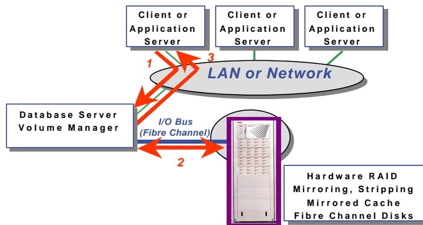
**Figure-4 (Server Attached Storage/Block or Fibre Channel Attached Database Model)**
