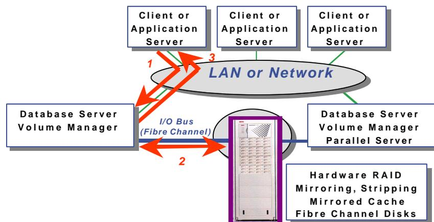
**Figure-5 (Redundant or Parallel Access Database Storage Model)**
